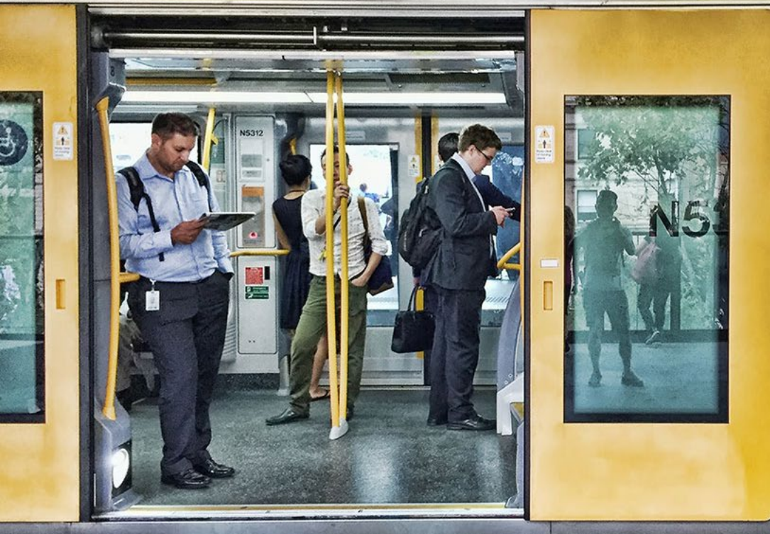
Extra-wide doors on Sydney's new Waratah trains allow for quick loading and unloading, which increases capacity.
